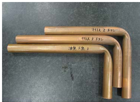
Degradation of sectional shape
